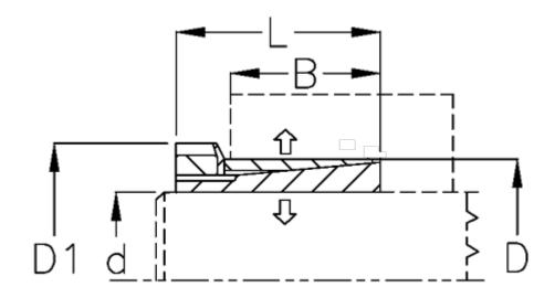
$\begin{array}{lll} \text{B mm} & = 22 \\ \text{D1 mm} & = 52 \\ \text{d H8 mm} & = 28 \\ \text{D mm} & = 40 \\ \text{Fit tolerance} & = \text{Aksel h8, Nav H8} \\ \text{F kN torque} & = 40 \\ \text{L mm} & = 35 \\ \text{P N/mm2 surface pressure on shaft/hub} = 110 \\ \end{array}$
